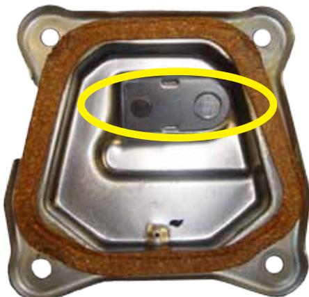
Externally the same, the bakelite valve of the T1 rocker cover has been replaced with a reed valve type on the T2. This was done to reduce noise primarily and has no effect on the performance of the engine. These parts are interchangeable.
