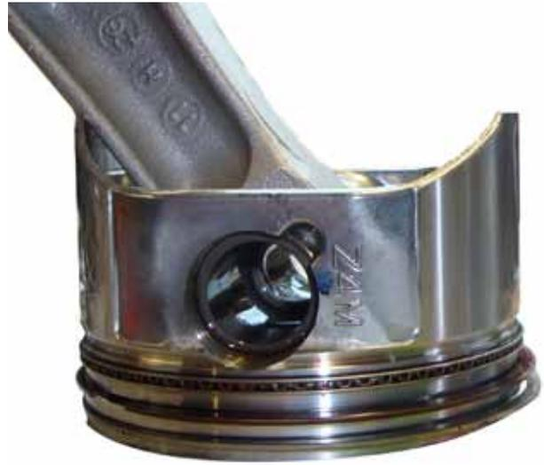
The T2 piston is shorter and has an additional curve under the oil ring. The top two piston rings are visually similar to the T1 but the oil control ring is thinner (2mm as against 2.5mm on the T1) and the ring groove in the piston is correspondingly smaller.
