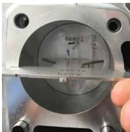
With the piston at BDC, the ABkC Block tool must sit flush on the deck face and be in line with the piston pin
