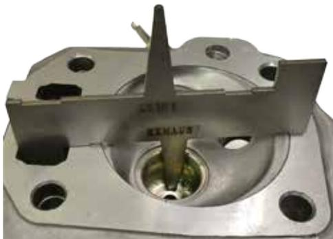
→ With the lug sitting on the land around the valve guide, the Inlet/Exhaust gauge must NOT sit flush on the cylinder head face, but rock
