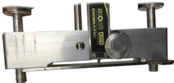
Using the CPO gauge to zero a caliper prior to its use for deck height measurements. Stroke can also be measured with this bridge
