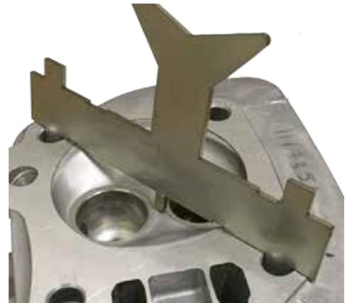
→ The spark plug insert must show a clearance to the CPO gauge, which must be flush on the cylinder face
