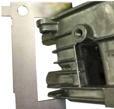
When placing the CPO gauge over the rocker cover face, the lower lip must not engage over the cylinder mating face
